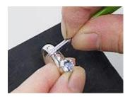
5) Polish the entire piece with a stainless steel brush, and make a mirror finish with a burnisher. Finally, polish using a polishing cloth with some metal polish.
