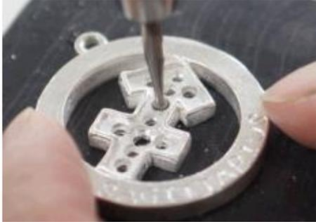
13) Fix the holes with a stone setting burr whose angle is the same as the curette angle of the round cut stone. This helps to set stones and prevents damage when making beading decorations with pressure.
