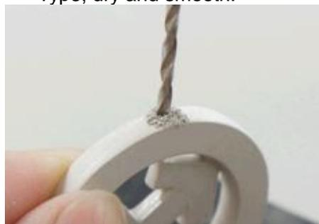
8) Drill a hole with  $\phi$  1.5 drill bit.
