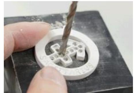
12) Drill a center hole with  $\phi$ 3 drill bit, and drill other holes with  $\phi$ 2 drill bit, and fire.
