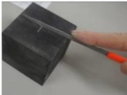
15. Cut  $\phi$  0.8mm silver wire into a 1cm length. Score both tips with the edge of medium fine file to attach firmly.
