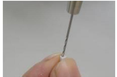
14. Smooth the surface with sponge sanding pads, and drill a hole into the piece with a  $\phi$  1mm drill bit.
