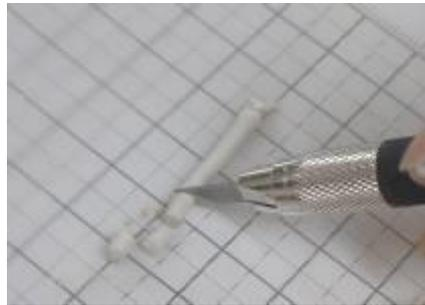
13. Cut the rope into 3pieces 5mm long with the craft knife. Make some spare pieces just in case.
